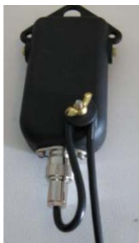
Balun Showing Coaxial Strain relief
