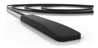
The 96ST008 is a unity gain, 3G Glass Mount Antenna suited for use in cellular bands PCS, GSM, UMTS, 3G & NEXT G. The antenna comes complete with 2.5 metres of low loss cable and an SMA male connector. The antenna is designed to be mounted on the inside of the vehicle front windscreen. The antenna operates through the glass.
